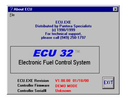
This screen gives the user our company information. This screen also allows the user to find out what version of ECU software is installed, and what version of firmware is installed in the engine controller. If technical support is needed on either the ECU System Console, or the engine controller, please reference the two printed revisions and have that information available for technical support.
