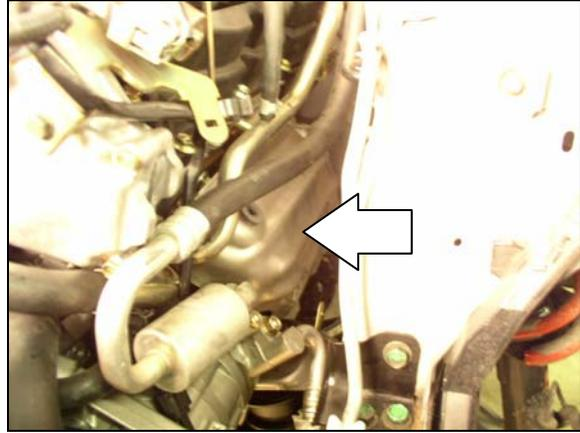
33. Re-install both halves of the upper intake plenum, as well as any removed hoses, clamps or electrical connectors, reversing steps 20 & 21. Don't re-install the plastic intake cover or strut tower brace at this time.
