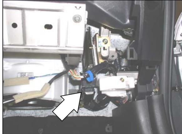
11. Once removed from the car, attach the Serial No. decal (P/N 31039) to the ECU in the location pointed out in FIGURE 8, and fill out the information on the label with a permanent black pen or thin-tip marker. **NOTE: All ECU's received with incomplete or illegible decals will be returned or discarded, so please print clearly and completely!**
