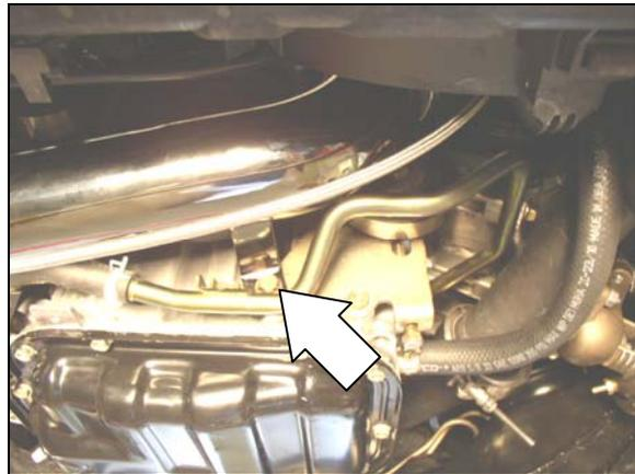
77. Install P/N 21176 (Tube Ass'y, I/C to MAFS 1) from the passenger side intercooler outlet to the tube from the previous step, using (1) 2-1/2" hump hose (P/N 30380-4) and (1) 2-1/2" coupling hose (P/N 30172-4) and (4) T-bolt clamps (P/N 30275-250), as seen in FIGURE 71. Use the coupling hose at the intercooler connection.
