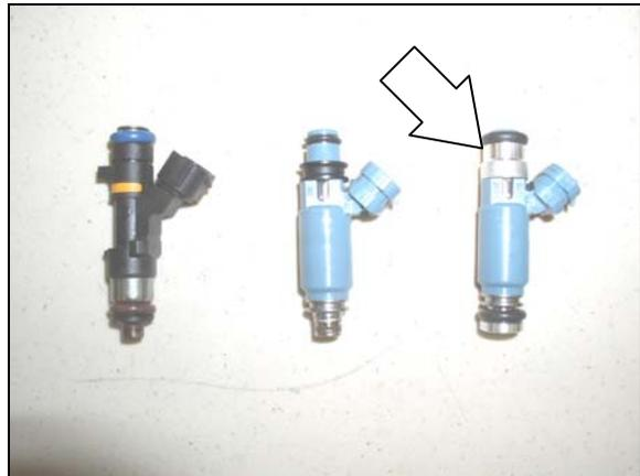
26. Sit down at a large open table, layout the 6 factory injectors and the 6 new injectors (P/N 31001) next to each other, and perform the following:
