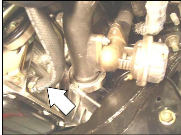
69. Install the third Downpipe (P/N 21201 or 21204, depending on which turbocharger system you purchased) using V-band clamp P/N 30232 to connect to the second downpipe, and (2) M10 x 40mm hex bolts, flatwashers, lockwashers & nuts to connect to the 2-bolt flange.
