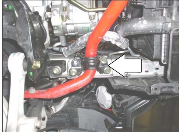
37. Remove front sway bar mounting brackets (shown in FIGURE 37) connected to the frame rail, so that the sway bar dangles loosely under the car. This step is optional, but makes the next few steps easier.
