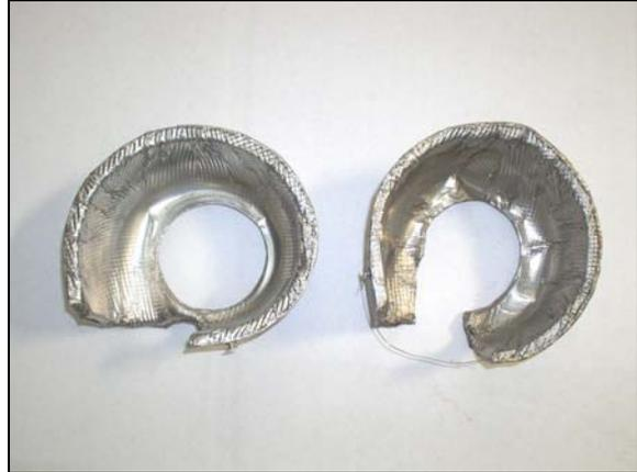
78. Modify P/N 30223 (turbo heat shield) as shown in FIGURE 72, using sheet metal cutters or heavy-duty scissors. Install the shield over the turbocharger turbine housing, and secure with steel wire.
