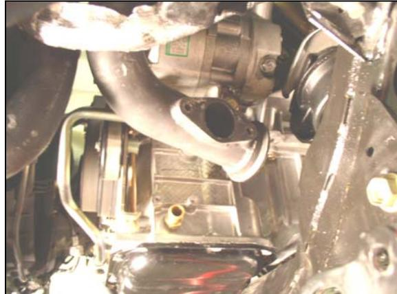
47. Either before or after loosely installing the "Turb. Housing Inlet" tube, install the "Turbo Support Bracket" (P/N 21202) circled in FIGURE 44, by loosening another of the A/C compressor bolts (on the driver's side top), and sliding the slotted end of the bracket under the loosened A/C bolt. The end of the bracket with the hole should line up with one of the holes in the turbocharger inlet flange (SEE FIGURE 44).
