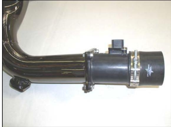
83. Loosen the factory bolt from the front side of engine, pointed out in FIGURE 76, and install the previous tube assembly using this bolt, and connecting to the 45-degree hose coupling from step# 76, and the tube in FIGURE 74. Reconnect the electrical connector to the MAFS housing (it may be necessary to cut a factory zip tie, to provide enough slack in the wire harness to reach the new MAFS housing location). Installed assembly can be seen in FIGURE 77.
