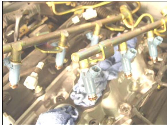
29. Re-install and bolt down both fuel rails, taking care while pressing each injector down into the lower intake plenum, to make sure each injector is properly seated on the injector spacers. Re-connect the electrical connectors to the injectors.
