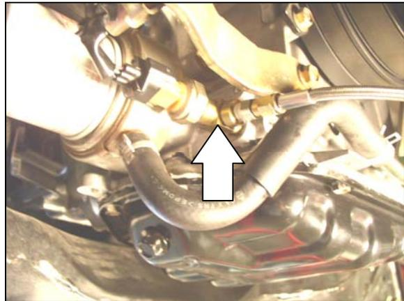
74. Install the mounting brackets (P/N 21203) to the intercooler end tanks, using (2) 1/4-20 x 1/2" hex bolts & lockwashers. Install the intercooler (P/N 5-312) assembly to the car using the factory bolts, as shown in FIGURE 65 & 66.
