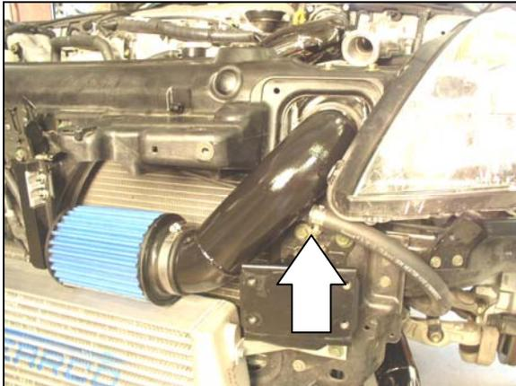
81. Install P/N 21179 (Tube Ass'y, MAFS to T/B) tube to the factory throttle body, using (1) 3.0" hose coupling (P/N 30162-4) and (2) T-bolt clamps (P/N 30275-300), as shown in FIGURE 74.
