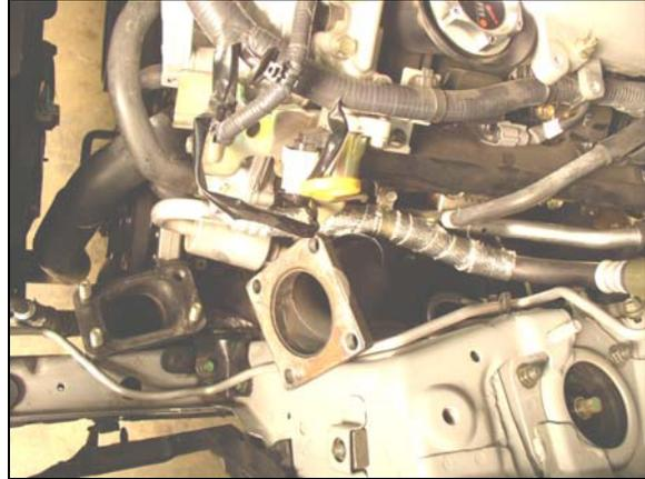
59. Install (3) M10 x 42mm studs and (1) turbine inlet gasket (P/Ns 30806, 30263) onto the turbine inlet flange as circled in FIGURE 53.
