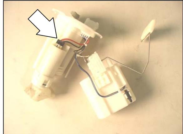
15. Sit down at a large open table, and prepare to disassemble the fuel pump assembly, per the following steps: (You will need a small flathead screwdriver, needle nose pliers, 7/64 and 3/8" drill bits and metal / wire cutters)
