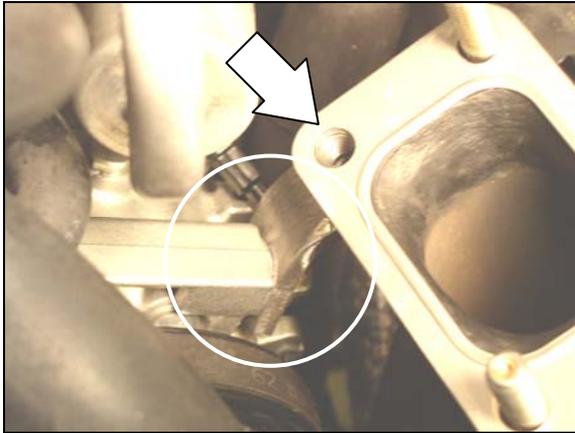
48. Install P/N 21183 (Exh. Tube Ass'y, Y-Pipe) into position shown in FIGURE 45, loosely securing it to the previous tube with v-band clamp P/N 30624.
