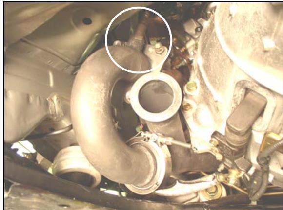
51. Install P/N 21186 (Exh. Tube Ass'y, Downpipe 2) into position shown in FIGURE 47, loosely holding it in position with steel wire, not fastened to anything. This is done now, because it is more difficult to install later in the instructions.
