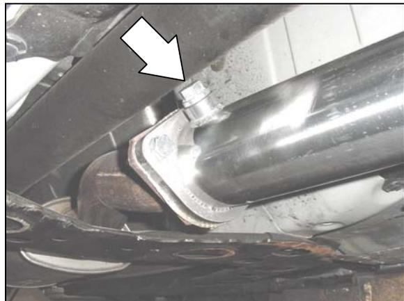
**NOTE:** Now that all exhaust tubes are loosely installed, go thru and tighten all the hardware & clamps.
