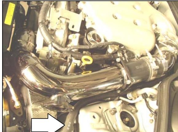
84. Install the polished discharge horn (P/N 20732P) into the discharge of the Raptor blow-off valve (P/N 10843) by simply pressing it into place. Mount the valve assembly to the swivel mount on the previous tube, using (1) O-ring (P/N 30468), and (2) 1/4-20 x 5/8" serrated head hex bolts. Orient the valve with the horn facing towards the front of the car and tighten the bolts.
