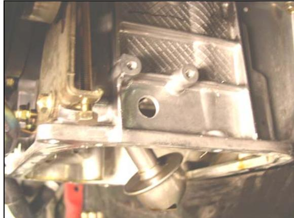
42. Deburr hole and thoroughly clean out any metal chips from inside of engine block. Install the 3/8" NPT x 5/8" hose barb fitting (P/N 30133), using NPT thread sealant tape.
