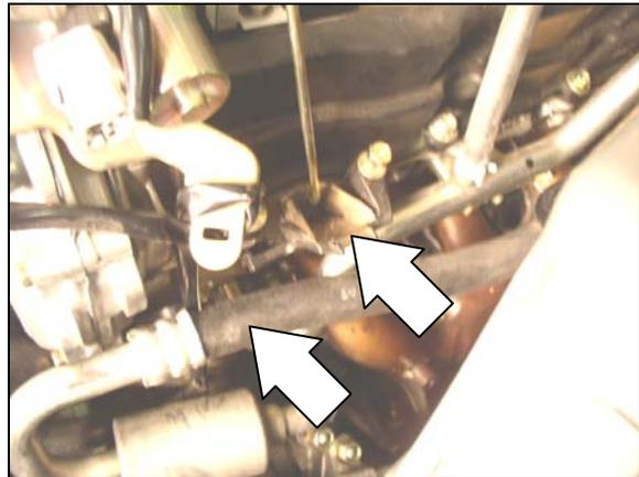
56. Wrap the A/C hose pointed out in FIGURE 50 with heat shield wrap (P/N 31007) as shown in FIGURE 51. You may want to secure the open end with a zip tie or steel wire.
