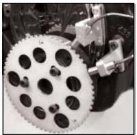
Small Chevy Bracket #210-72701 on timing cover & #210-72802 New 30° Bracket on front motor mount which works well on late models (Vortec etc.), or as back-up sensor. Also use both with GM Odd-Fire 4.3 Liter based V-6's.
